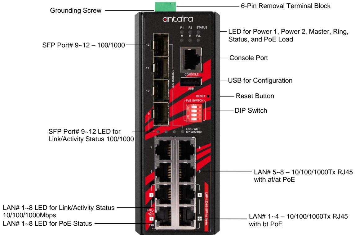
*Figure 2.2 - The Front Panel of LMP-1204G-SFP-bt Series*
