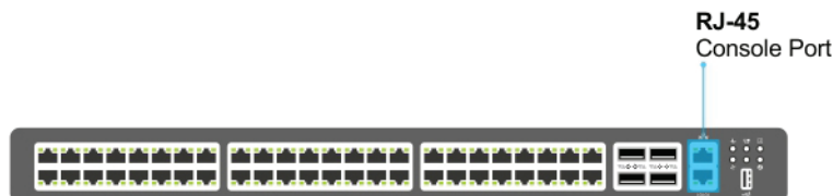
FIGURE 8-1. SWITCH RS-232 CONSOLE PORTS
