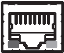
Figure 3-10. CATx connector.
