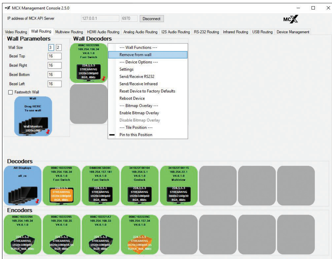
FIGURE 4-9. REMOVING A DECODER (RX) FROM A WALL
