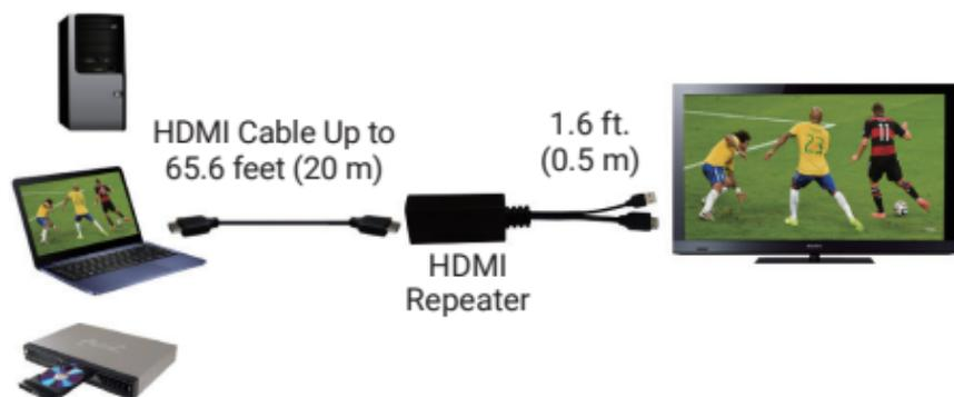
The HDMI Repeater extends an HDMI signal up to 65.6 feet (20 m) via a high-speed HDMI cable connected to the video source and built-in HDMI and USB cable connected to the HDMI 4K @ 60 Hz display.
