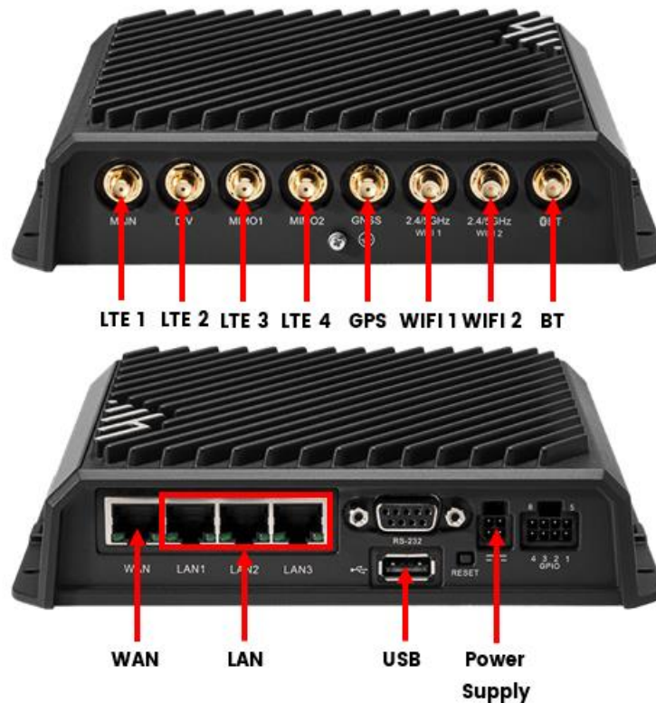
Figure 8: Cradlepoint R1900 Connections
