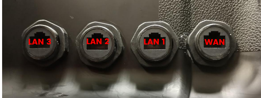
Figure 9: Connect the router to the RJ-45 ports on the case using ethernet cords.
