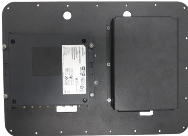
Figure 4: For R1900 router, fasten the router to the cover plate using PTA0579 screws and PTA0604 nuts.
