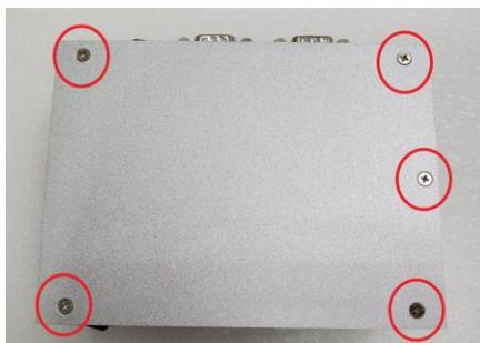
**Step 3** Open the bottom cover and locate the memory module.
