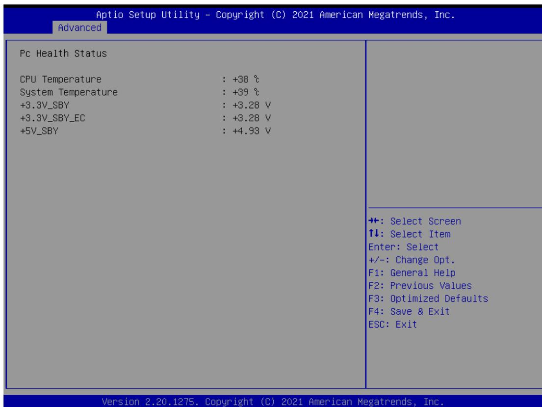
This screen displays the temperature of system and CPU, system voltages (VBAT, +3.3V, +3.3V standby and +5V).
