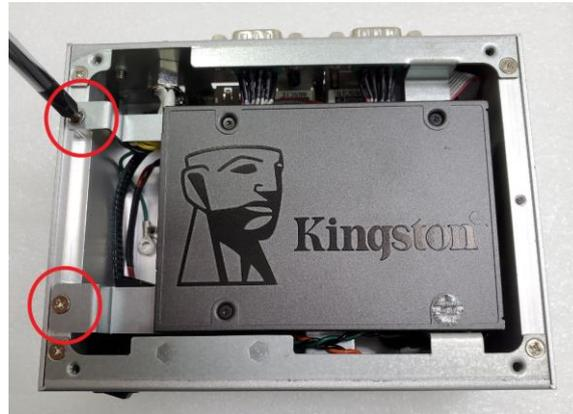
**Step 6 Put the bottom cover back and fasten all of screws.**
