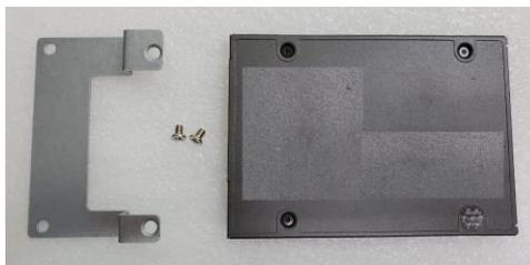
**Step 4** Assembly the SSD/HDD with the two HDD mounting screws and connect the SATA cable. Be sure the PCB side of the SDD/HDD facing to left.
