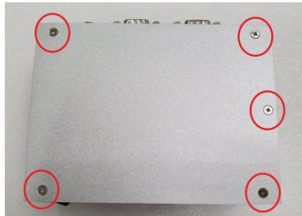
**Step 3** Open the bottom cover and prepare the SSD/HDD and bracket from the accessory box.
