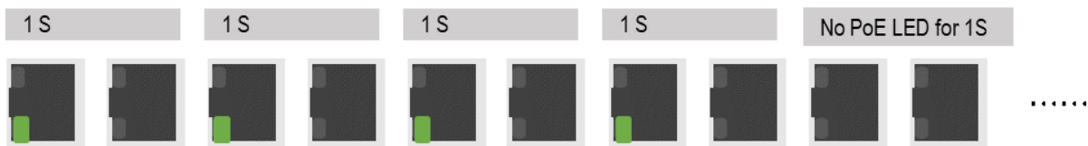
Figure 2.6 - PoE Over Current Recovering LED Sequence
