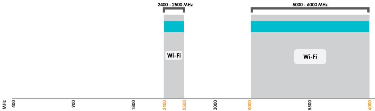
Indicates the WI-FI bands on which Heli-41 works
