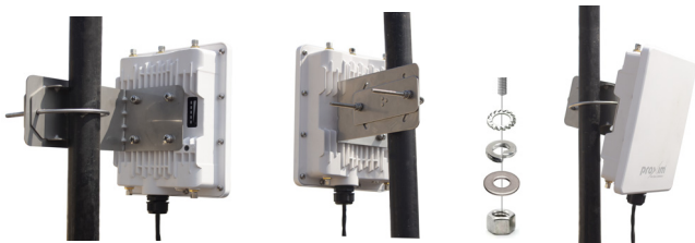
Figure 4: Pole Mounting
