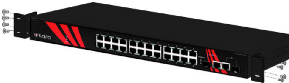
Figure 3.1 - Attach Mounting Plates with Screws
