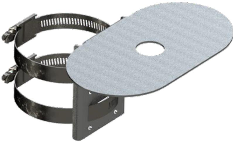
This bracket is designed for smaller antennas needing a 1-inch mounting hole. The included adjustable gear/worm-drive clamps fit poles or rectangular posts with 2.5 to 3.5-inch widths. Slots for gear clamps run vertically and horizontally.
