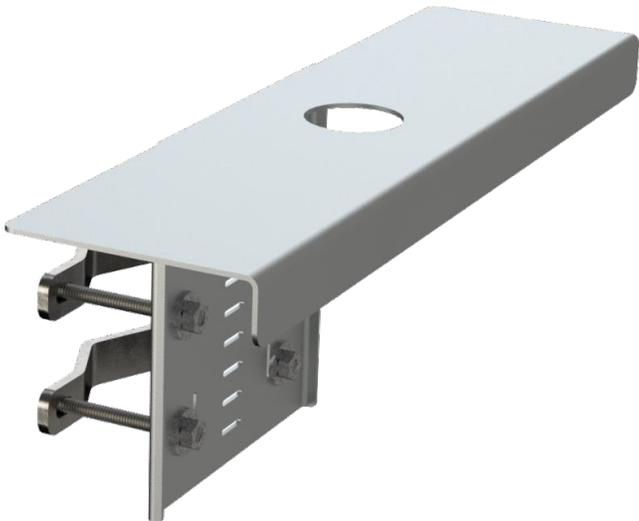
This bracket with a 14-inch-long plate is designed for longer antennas needing a 1.5-inch mounting hole. Bracket is designed to securely fit poles with 1 to 2.18-inch diameters or rectangular posts up to 3 inches wide. Additional slots for gear/worm-drive clamps run vertically and horizontally.
