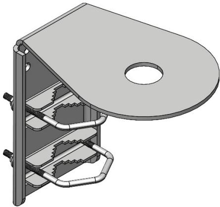
This bracket is designed for antennas needing a heavy-duty mount. This bracket has had stiffeners removed, removing stress concentration points and is twice the thickness of the PTA0149 mount. This Bracket is designed for antennas needing a 1.5-inch mounting hole to securely fit poles with 1.5 to 2.5-inch diameters.
