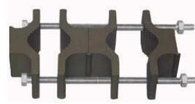
**BSLLUMNT 2-4** Dual Heavy Duty Base Station Mount. The BSLLUMNT2-2 mount is the double mount version of the BSLLUMNT1-2 that is designed to be used with BSLXL and BSLLXL series base station antennas. The mounts each consist of 4 extruded aluminum brackets and 2 8" Galvanized 5/16" 18THD bolts washers and nuts that will handle a 3" diameter mast.
