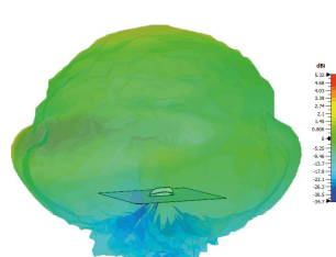
Typical 3D Pattern Elements 5 600x600mm 5.4GHz*
