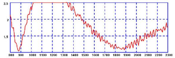
\* VSWR measured with 5m of CS29 cable on a 300x300mm (1' x 1') ground plane
