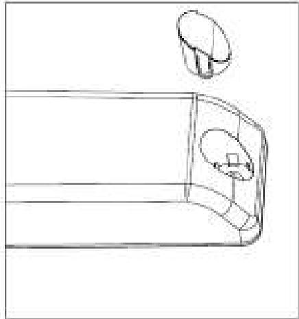
2 ONCE THE ANTENNA HAS BEEN SCREWED ONTO THE WALL, PUSH THE LOOSE SNAP FIT HOLE COVERS INTO THE TOP AND BOTTOM SCREW HOLES.
