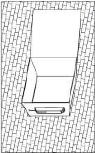
1 FOR EXTERIOR WALL MOUNTING AND METER BOX INSTALLATIONS USE STEP 1 & 2 FROM INTERIOR MOUNTING BUT MAKE SURE THE ADHESIVE PAD IS USED FOR SEALING PURPOSES. SMA CABLE CAN BE RUN DOWN THE BACK OF THE METER BOX OR OUT THROUGH AN EXIT HOLE.
