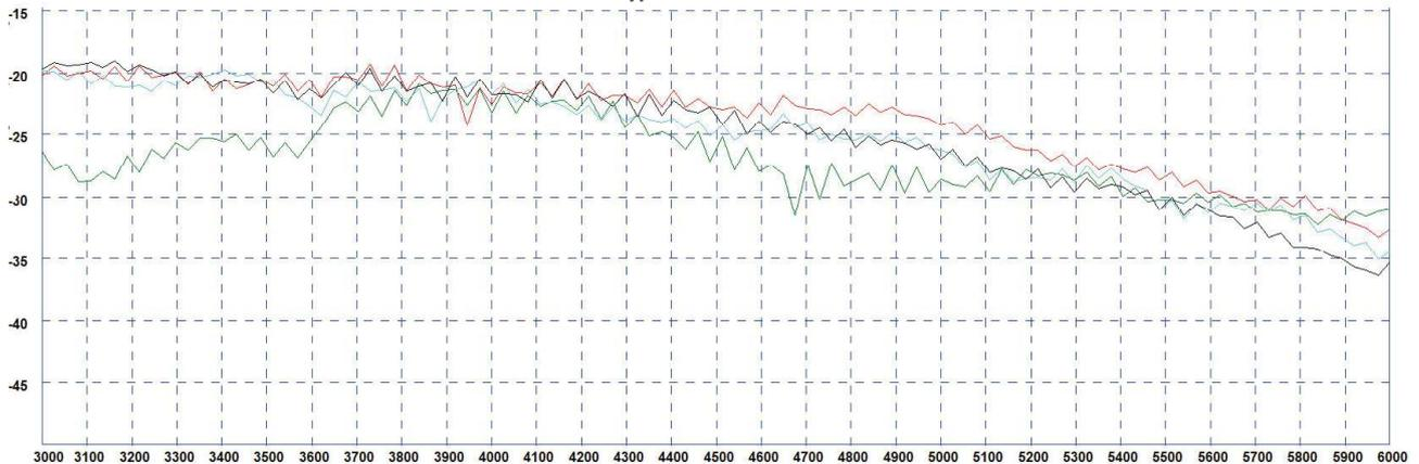
\*Typical Isolation measured with 2m RG174 cable in free space Red Trace = elements 1-2 Green Trace= Elements 1-3 Blue Trace = Elements1-4 Black Trace = Elements 2-3
