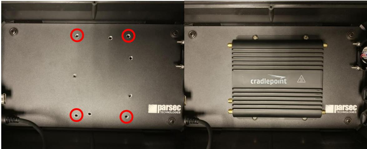
*Figure 3: Fasten the router to the bottom plate using PTA0399-TL screws.*
