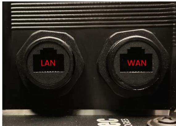
*Figure 7: Connect the router to the RJ-45 ports on the case using ethernet cords.*
