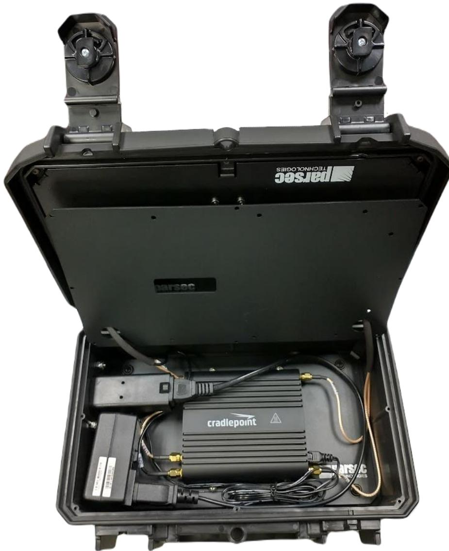
Figure 9: Fully Connected 5in1 Golden Retriever A with Cradlepoint IBR900 Router
