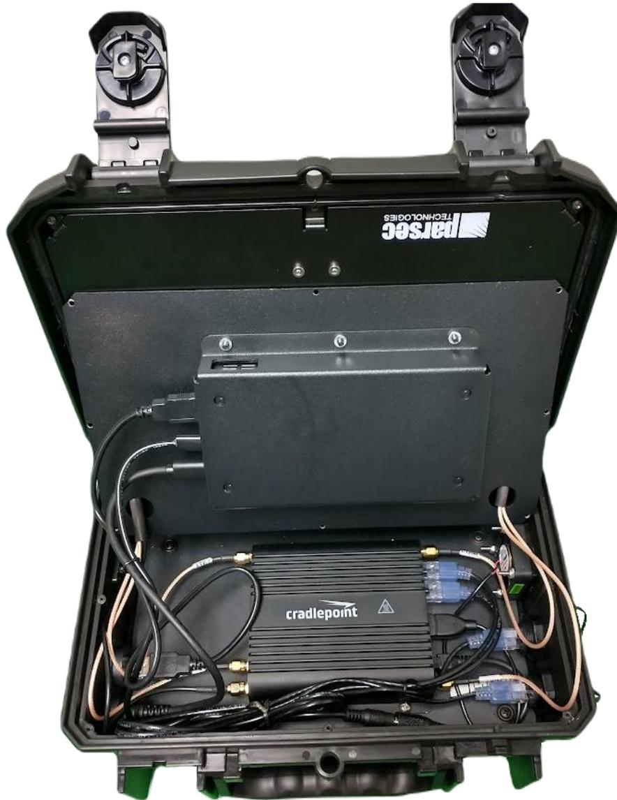
*Figure 10: Fully Connected 5in1 Golden Retriever G with Cradlepoint IBR900 Router*
