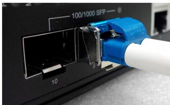
*Figure 2.9 - LC Connector to the Transceiver*
