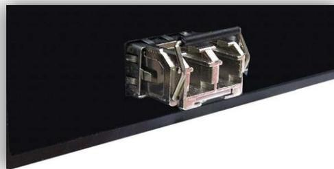
Figure 2.6 - Transceiver Inserted
