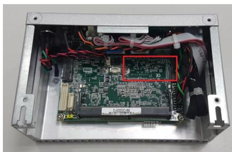
**Step 5** Insert the M.2 SSD module firmly and secure the screw.
