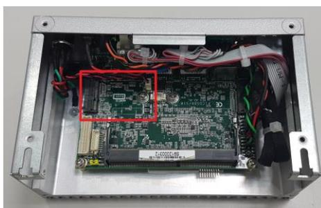
**Step 5** Insert the M.2 WiFi module firmly and fasten the screw.
