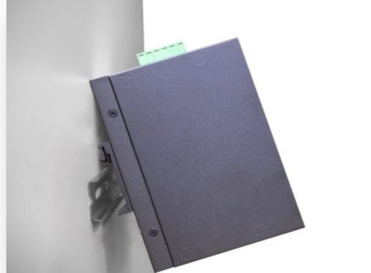
Figure 3.3 Stable the Switch on DIN-Rail
