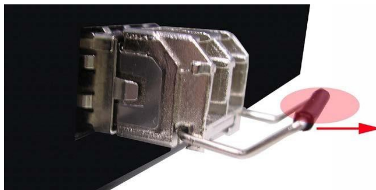
Figure 2.11 Pull Out from the SFP Module
