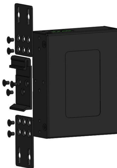
Figure 3.4 Remove DIN-Rail Bracket
