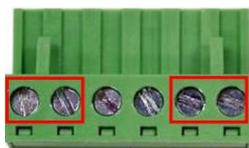
Figure 2.8 - Power Terminal Block
