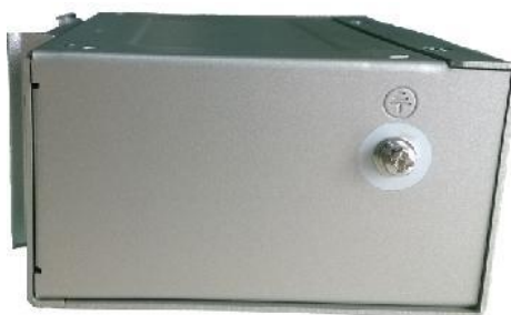
Figure 3-6. The grounding screw.
