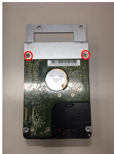
Figure 2-6 Fastening a HDD to the bracket
