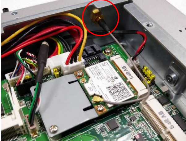
Figure 2-14 Antenna outlet (internal view)
