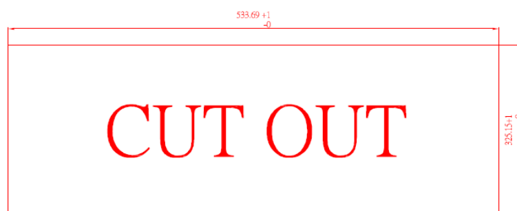
Diagram 1-3 Cutting-out dimensions of the GOT3217WL-845-PCT
