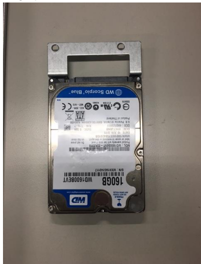
Figure 2-6 Fastening a HDD to the bracket
