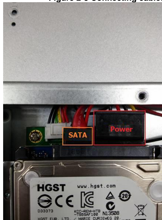
Figure 2-8 Connecting cables to connectors
