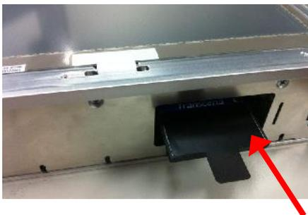
**Step 4 Close the cover of CF card slot and fix it. Installation completes.**
