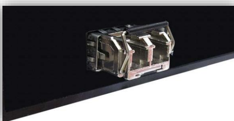
Figure 2.8 - Transceiver Inserted
