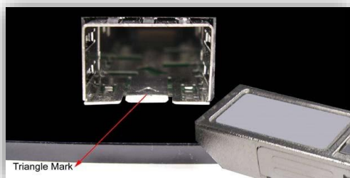
Figure 2.7 - Transceiver to the SFP Module
