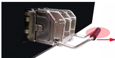
Figure 2.11 - Pull Out from the SFP Module
