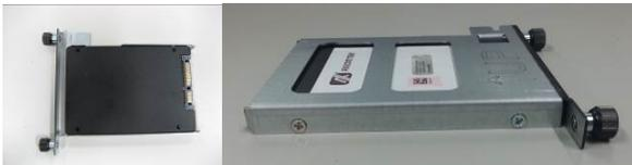
**Step 3** Slide CFast card or HDD/SSD into slot carefully
