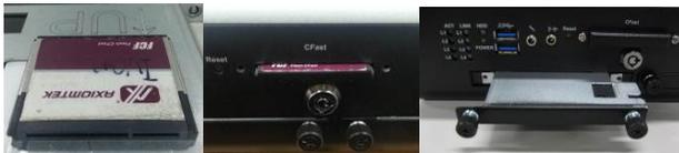
**Step 4** Fasten screws of HDD/CFast bracket
