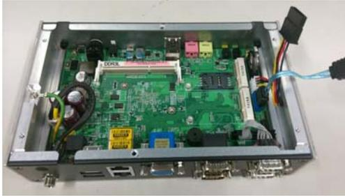
**Step 3** Locate the memory module, insert the gold colored contact into the socket.
