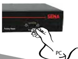
Connect the host PC and PS810's console port using a serial console cable.
