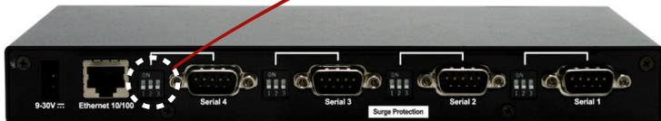
Set serial DIP switch according to your serial device requirements(RS-232/422/485)
