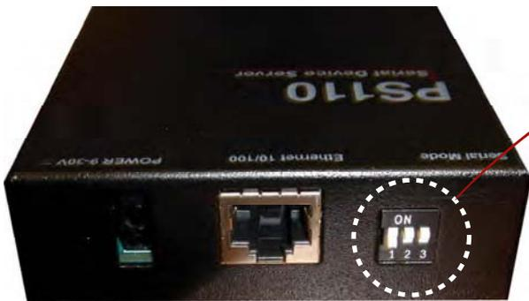
Set serial DIP switch according to your serial device requirements(RS-232/422/485)
