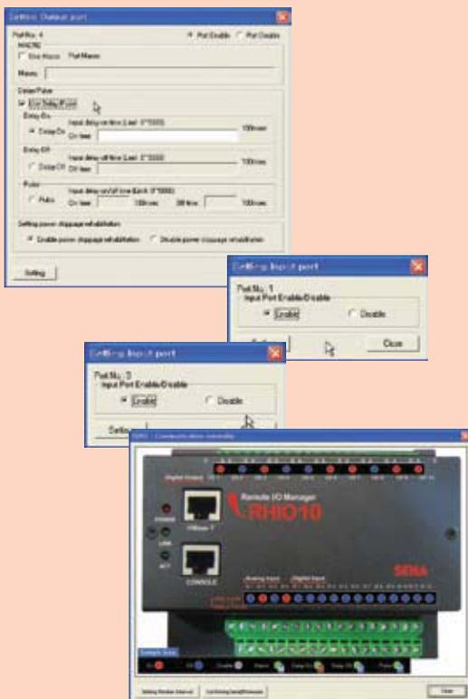
**The Rhio10**, Remote I/O Manager is simple and easy-to-use Ethernet Data Acquisition System that communicates with PCs and other computers over Ethernet and Internet networks. They utilize the open systems environment of Ethernet to acquire data from any number of remote locations.
