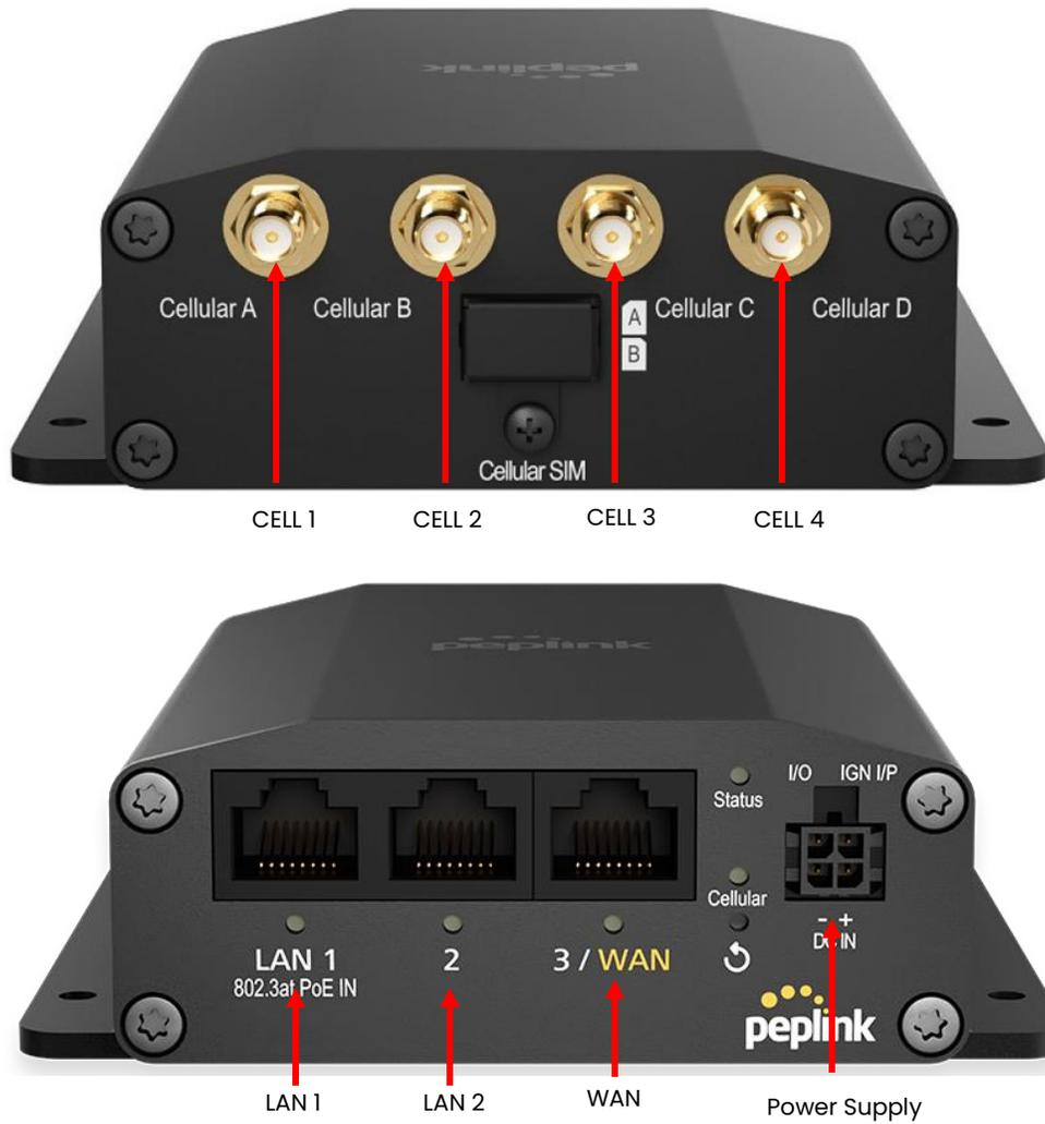
Figure 8: Peplink MAX BR1 Mini 5G Connections
