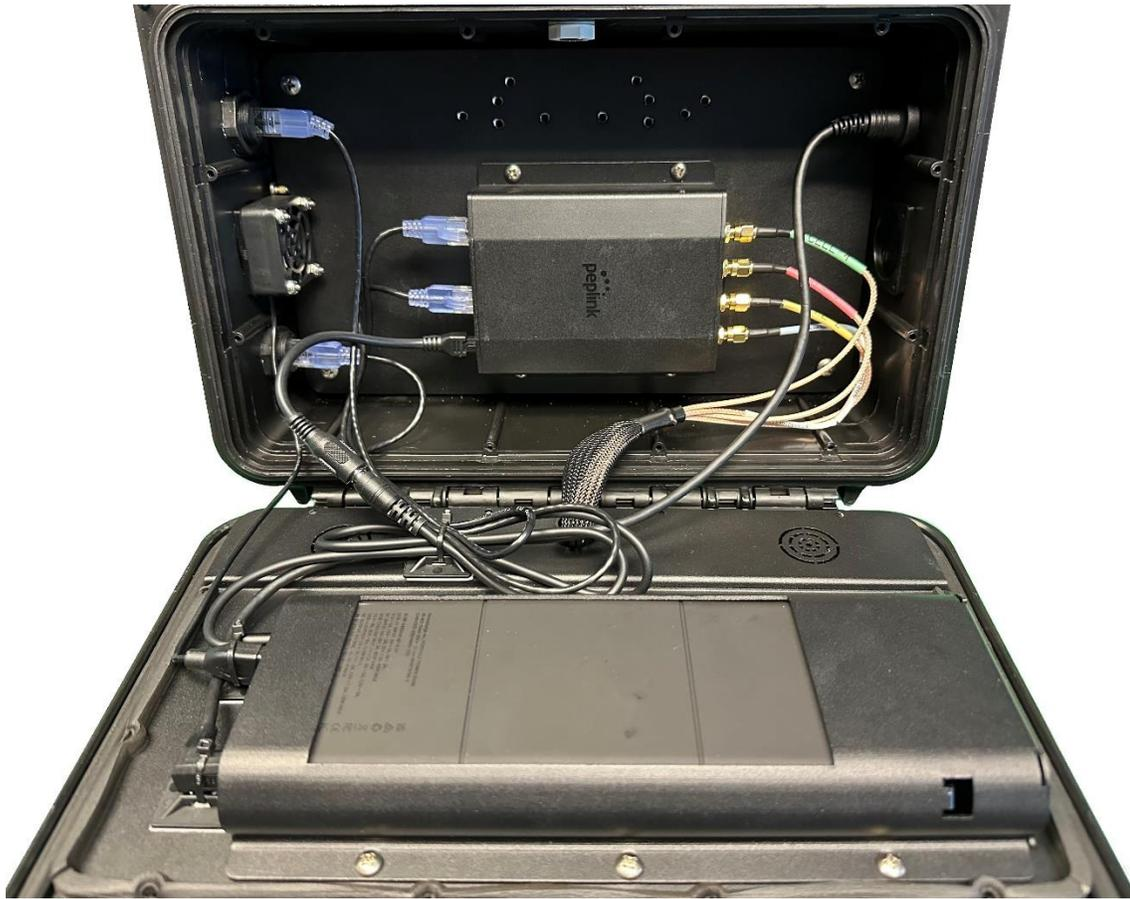
*Figure 17: Fully Connected 4in1 Boxer G2 with Peplink MAX BR1 Mini Router*
