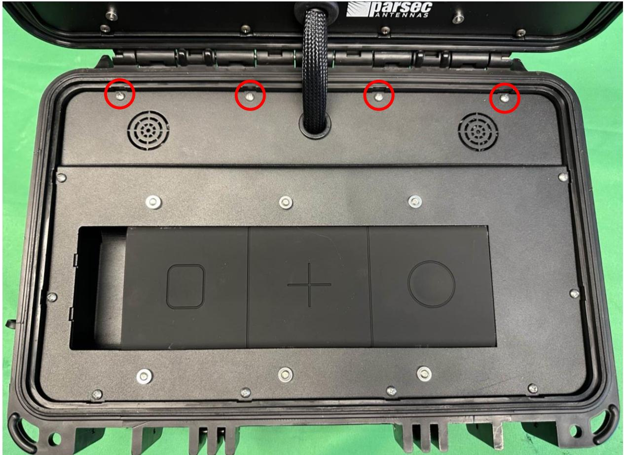
*Figure 20: Fasten the cover plate to the case using PTA0071 screws.*
