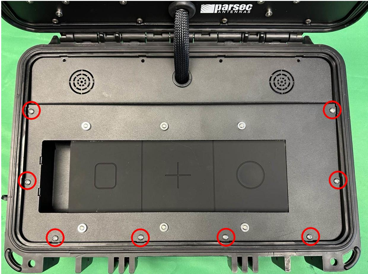
*Figure 19: Fasten the cover plate to the case using PTA0099 screws.*
