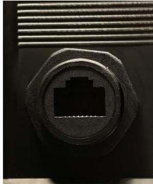
Figure 9: Connect the router to the RJ-45 ports on the case using ethernet cords.
