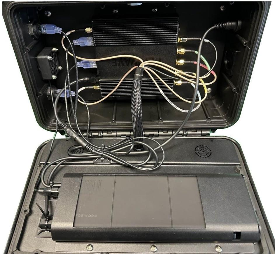
*Figure 16: Fully Connected 7in1 Boxer G2 with Peplink MAX BR1 Pro 5G Router*
