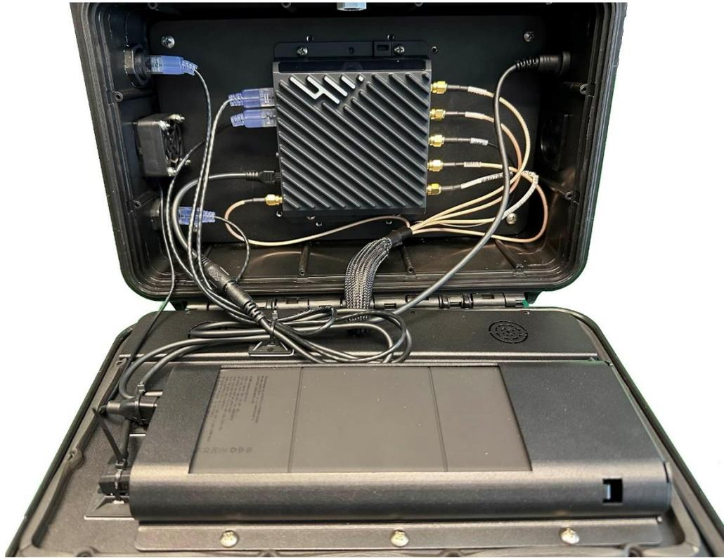
*Figure 15: Fully Connected 6in1 Boxer G2 with Cradlepoint R920 Router*
