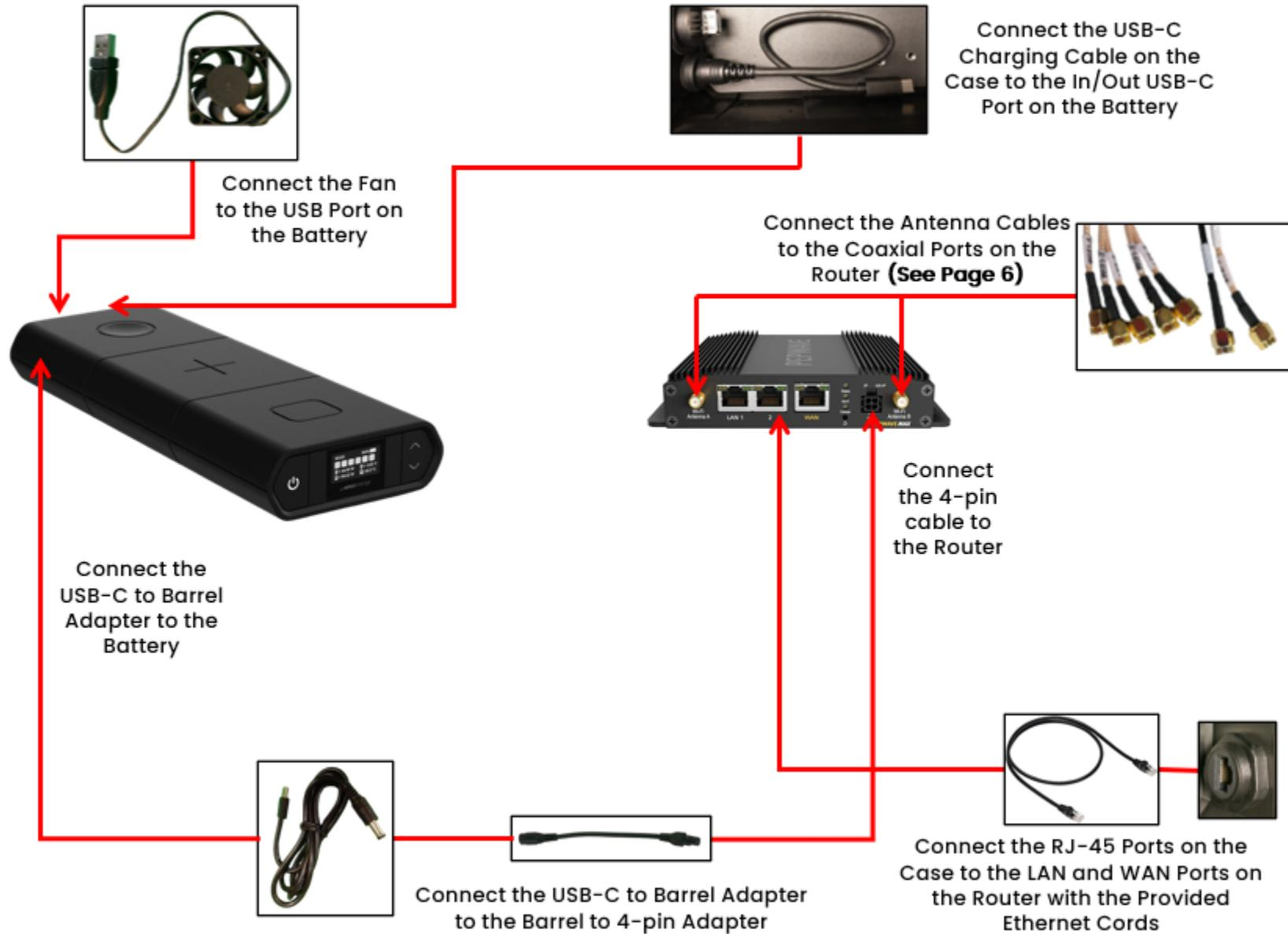
Figure 4: Connection Diagram for Boxer G2
