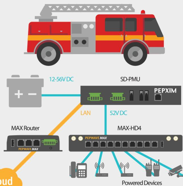
For unbreakable remote access to the SD-PMU, a secondary router can be connected to the LAN port. That way, the SD-PMU is accessible even when the main router loses connectivity. An additional benefit is that power to the main router could also be remotely scheduled from the IoT cloud.
