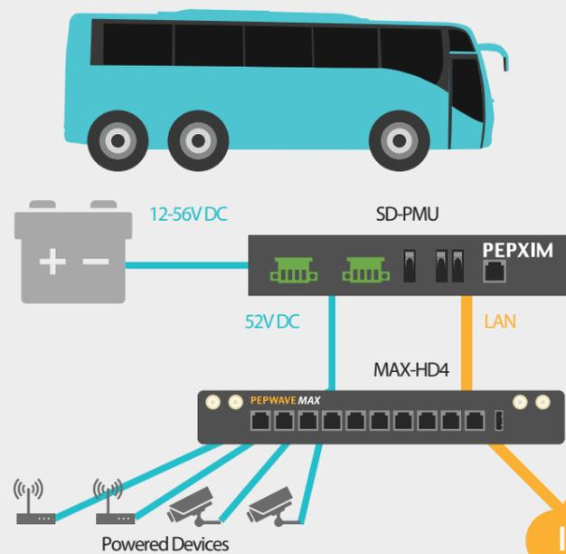
Connect the SD-PMU to your car battery to deliver reliable 52V power. Connect the LAN port to your router in order to remotely monitor battery output via the IoT Cloud. With 52V power delivery, the SD-PMU can support switches with 802.3at PoE output.
