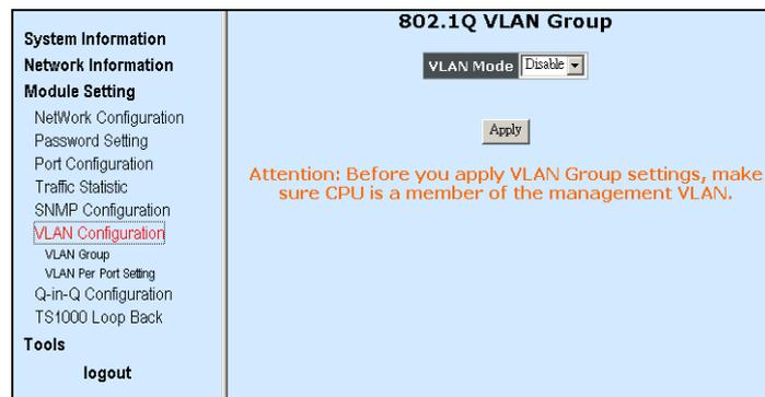
**VLAN Group:** To enable or disable VLAN Mode. When enabled, you can further indicate a VID to the selected ports.
