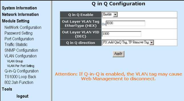
Step 1. By default, Q-in-Q is disabled. Make sure Q-in-Q is enabled before apply the settings.
