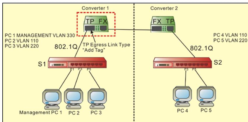
Step 2. Set FX port's Egress Link Type to "Don't Touch Tag". When PC2 wants to send a frame to PC4, the Converter will forward it out FX port directly based on settings in "802.1Q VLAN Group".
