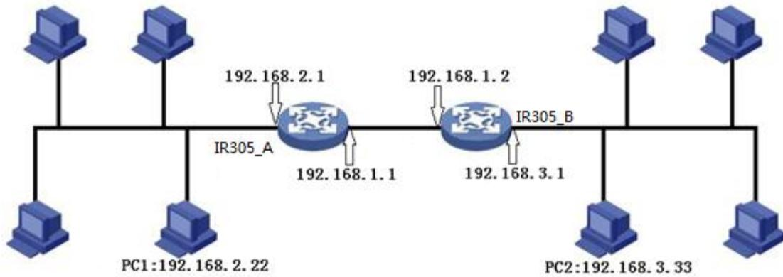
1 Configure IR305\_A. Click “Network >> OSPF” to access to OSPF configure page. “Router ID” should be in the same segment to IR305\_B. Configure IR305\_A in “Network” bar to announce the routing entry of the device.
