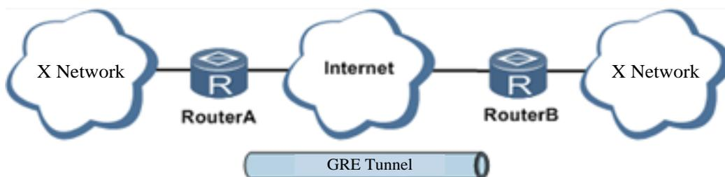
Along with the extensive application of IPv4, to have messages from some network layer protocol transmitted on IPv4 network, those messages could be encapsulated by GRE to solve the transmission problems between different networks.
