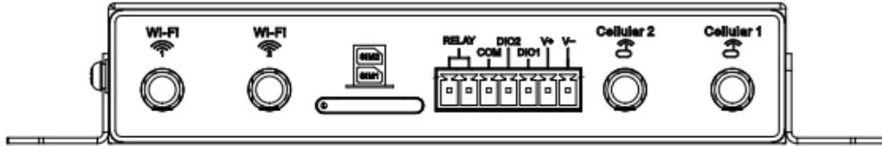
Wi-Fi antenna    Sim card slot
