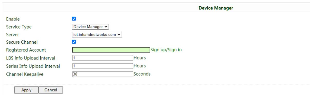
Login your account in Device Manager, and add your device in "Gateways", named your device and fill in the serial number from device, then you can manage your router in DM.
