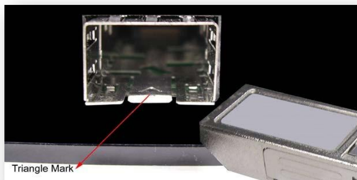
Figure 2.9 - Transceiver to the SFP Module
