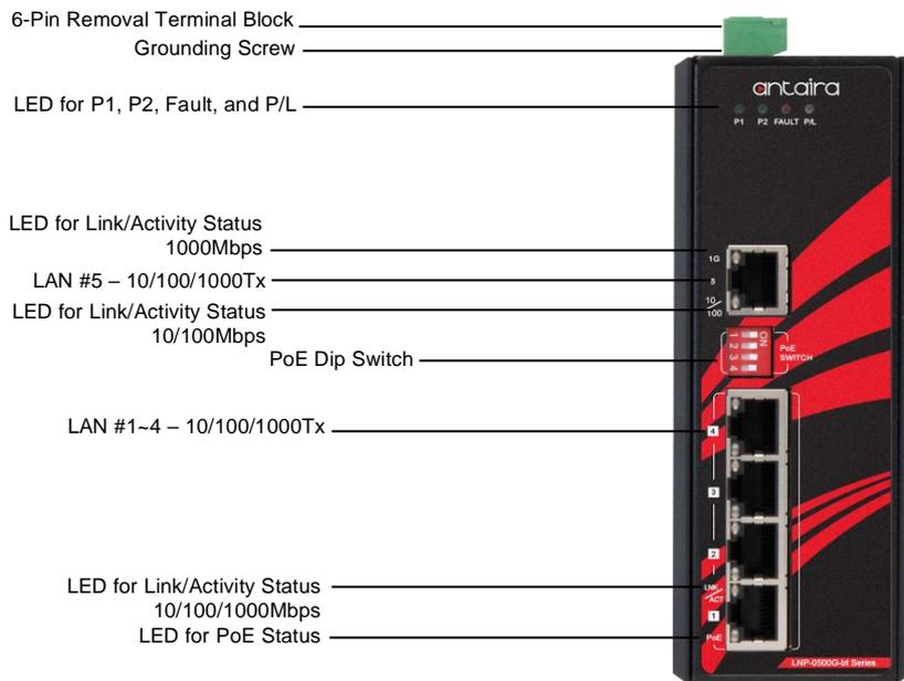
Figure 2.2 - Front Panel of the LNP-0500G-bt Series
