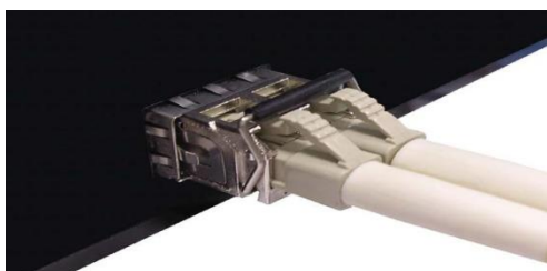
Figure 2.7 - LC Connector to the Transceiver
