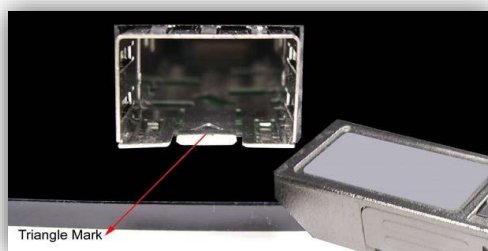
Figure 2.5 - Transceiver to the SFP Module
