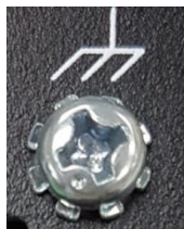
Figure 2.15 - Grounding screw
