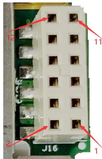
Note: the signals of Ethernet port are without magnetics.
