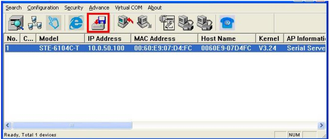
And then the user can select and download the required firmware from the disk, as shown in the figure below. The user can also select several same devices at one time, and realize the firmware updating for them by selecting **Apply for all selected devices have same model**.
