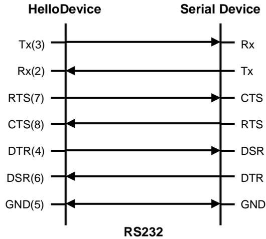
Figure A-6 RS232 wiring diagram
