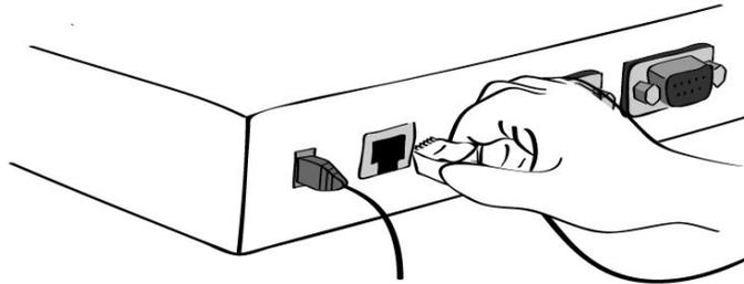
Figure 2-5 Connecting a network cable to the PS410
