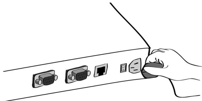
Figure 2-12 Connecting the power to the PS810
