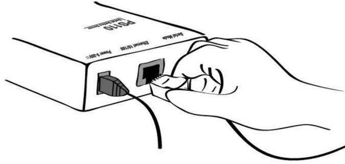
Figure 2-4 Connecting a network cable to the PS110
