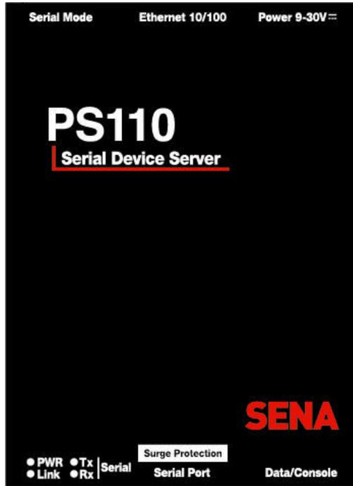
Figure 2-1 The panel layout of the PS110
