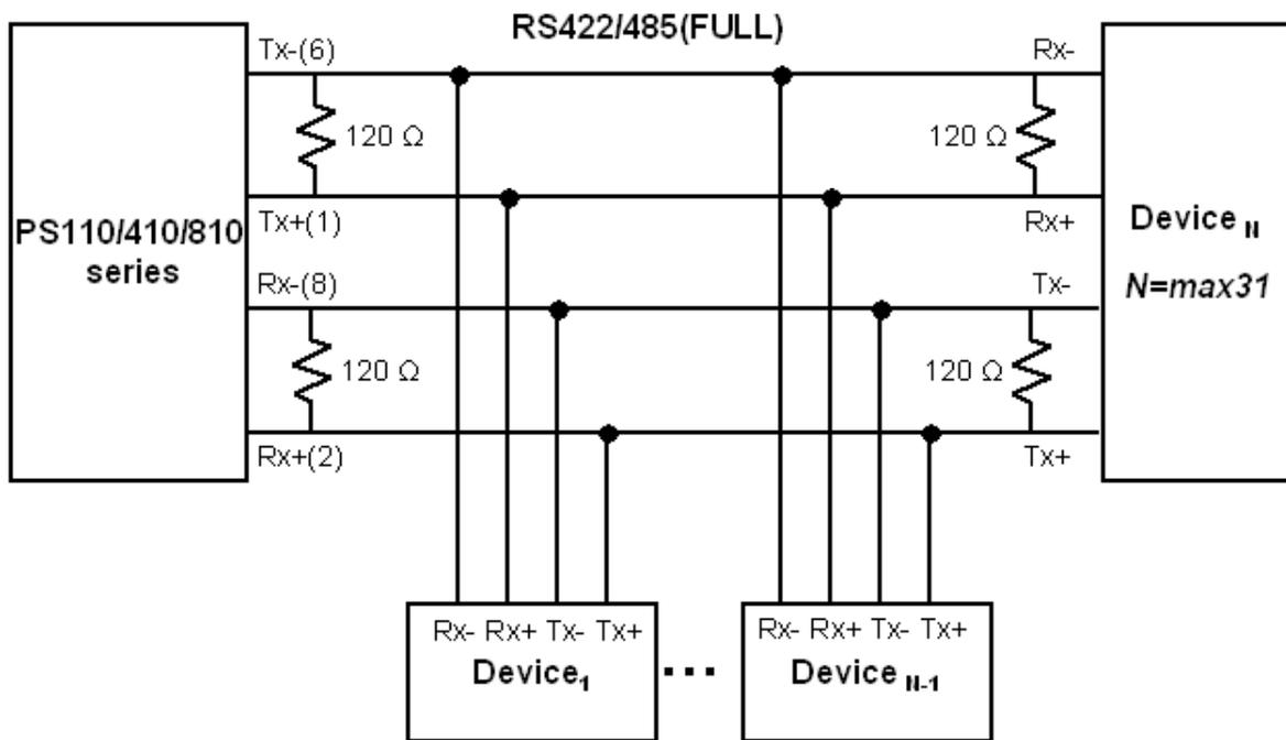
\* Termination Resistor at Tx side can be omitted if the signal status is good.
