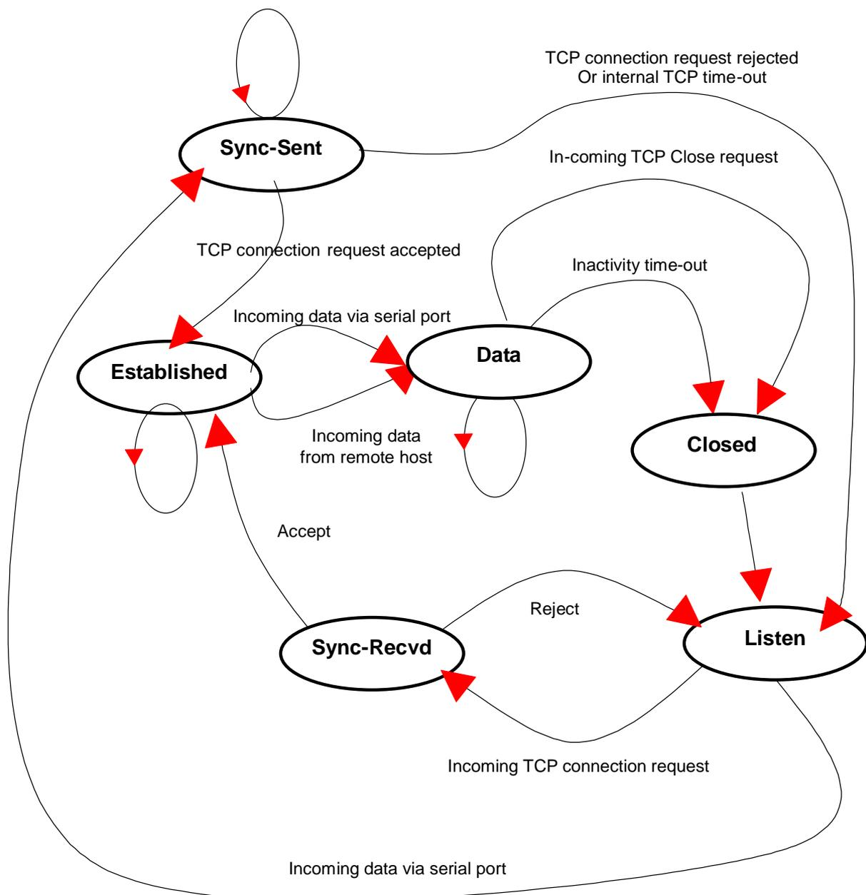
Figure 4-5 State Transition Diagram of TCP mode
