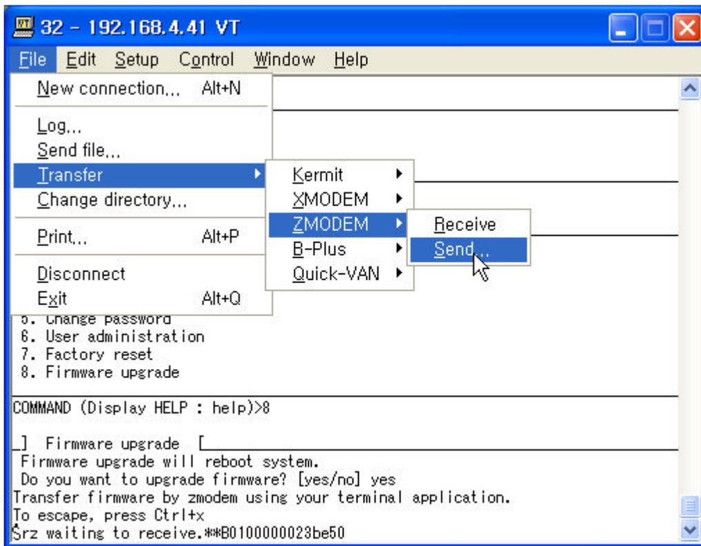
Figure 5-11 Transfer binary file by Zmodem (TeraTerm Pro)
