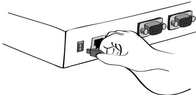
Figure 2-11 Connecting the power to the PS410
