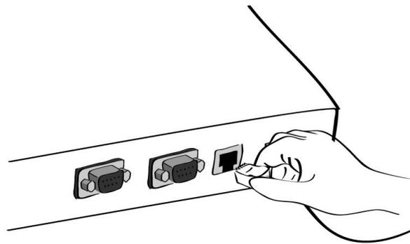
Figure 2-6 Connecting a network cable to the PS810
