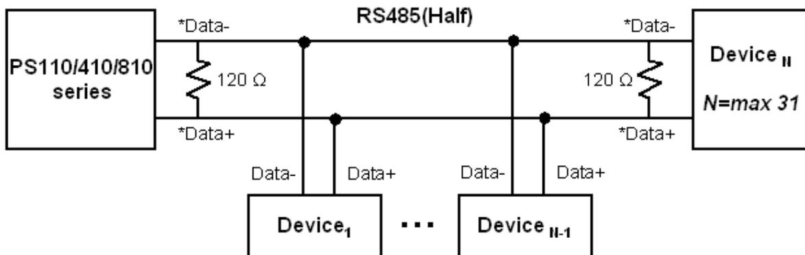
\*Data+ means that coupling of Tx+(1) pin and Rx+(2) pin
