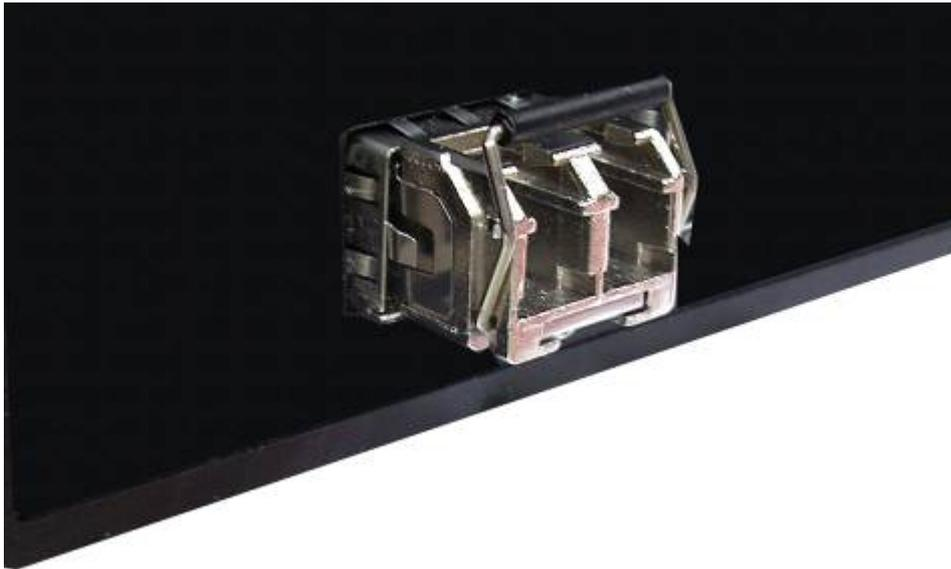
*Figure 2.9: Transceiver Inserted*
