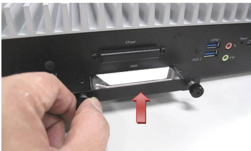
**Step 7 Fasten screws of HDD bracket**
