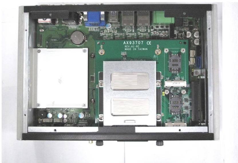
**Step 4 Slide Mini card into Mini Card slot with caution, and fasten screw of Express Mini Card.**
