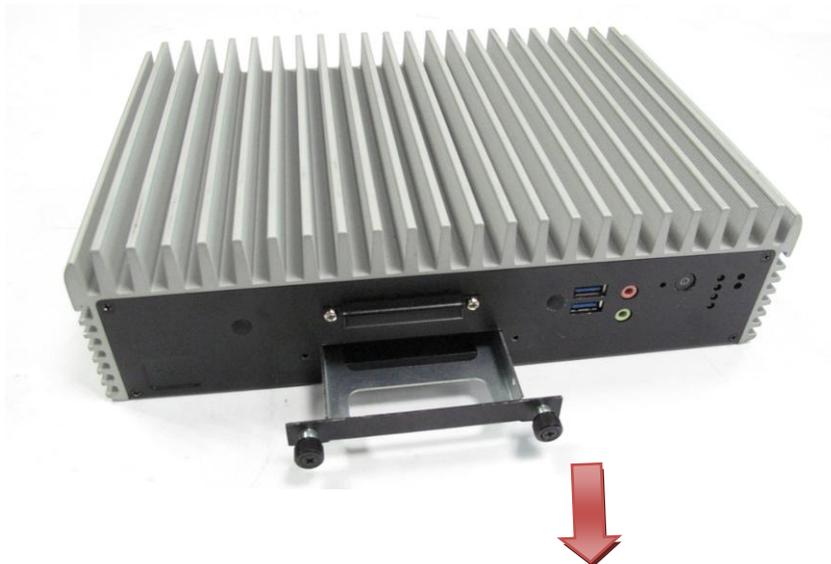
**Step 5 Assembly the HDD bracket together with the 2.5" SATA device**
